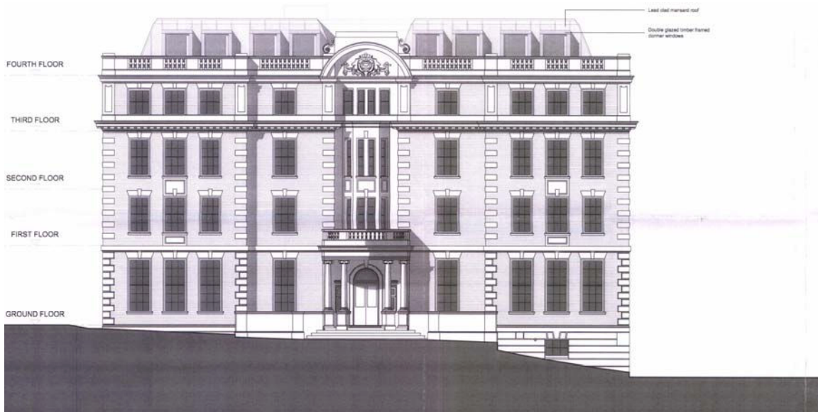
Proposed Front Elevation (Showing roof addition)
